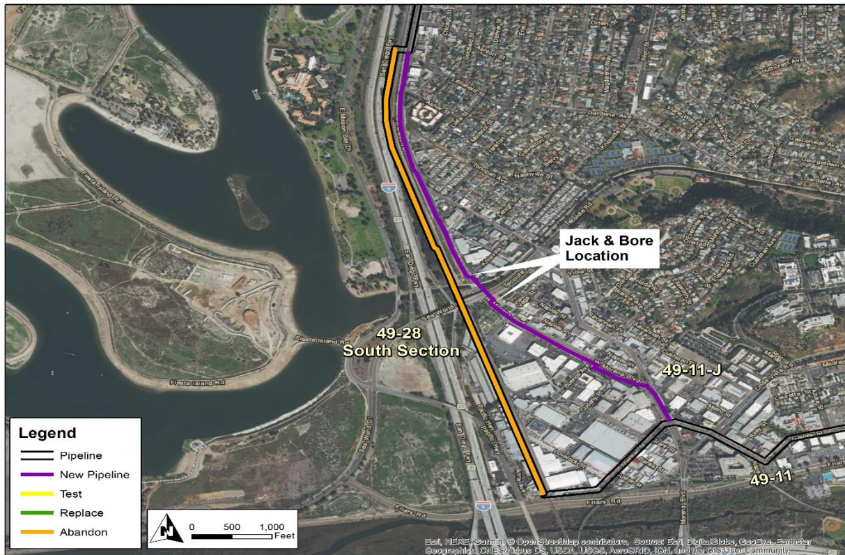
Figure 3: Satellite Image of Supply Line 49-28 South Section Replacement Project
